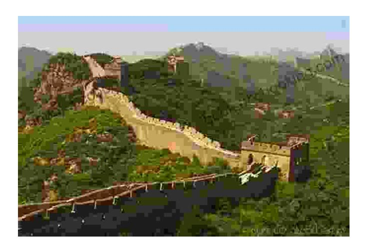
The Great Wall of China is a remarkable feat of engineering and construction. Its walls are made of tamped earth, stone, and brick, with watchtowers and fortresses strategically placed along its length. The wall's height and width vary depending on the terrain, with some sections reaching heights of over 25 feet.
